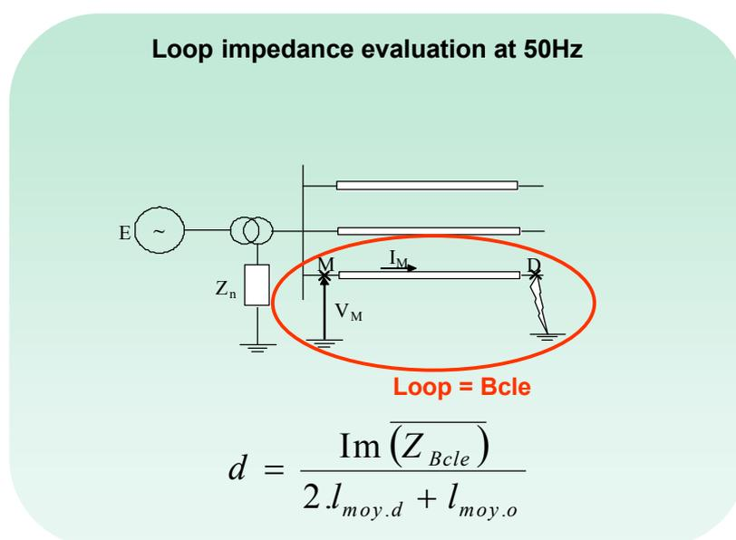
Figure 6-2 Loop impedance used for fault distance evaluation
