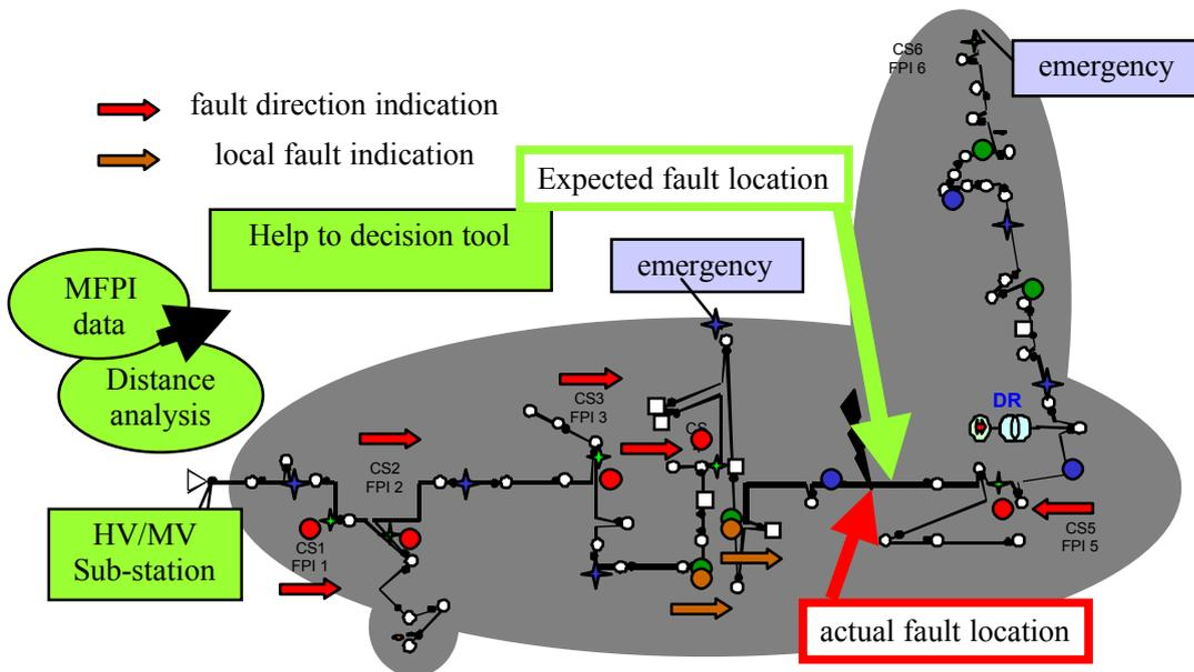
Figure 6-5 Fault localization principles step 2: the fault is cleared and investigated
