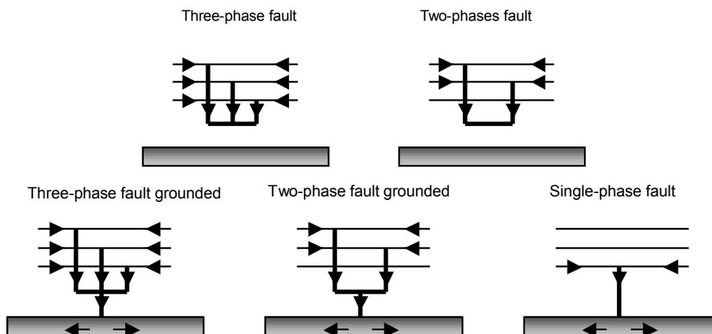
Figure 2-1 Fault types
