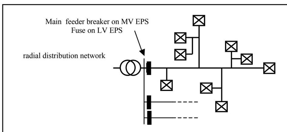
Figure 3-2 Distribution EPS operated in a radial topology
