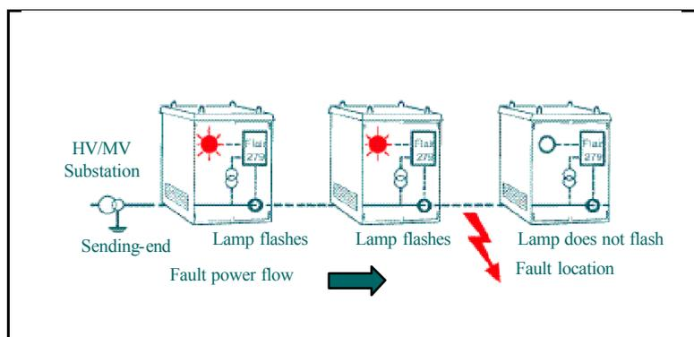
Figure 4-1 Non-directional FPI principle
