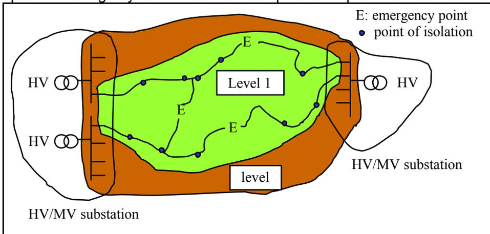
Figure 3-4 level 1 cell and level 2 cell principle
