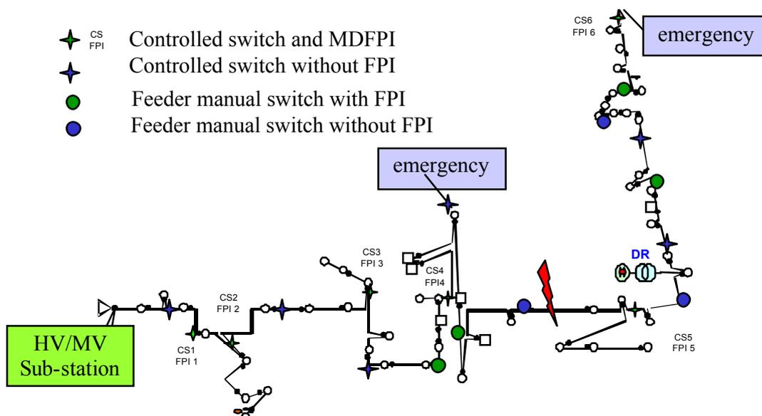
Figure 6-4 Fault localization principles step 1: a fault occurs
