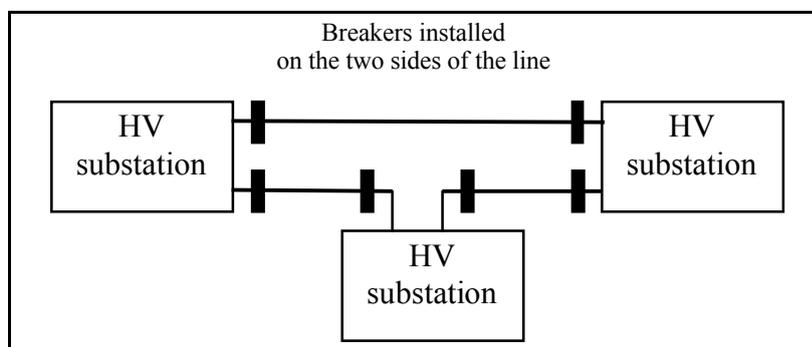
Figure 3-1 Transmission EPS operated in a loop or meshed topology
