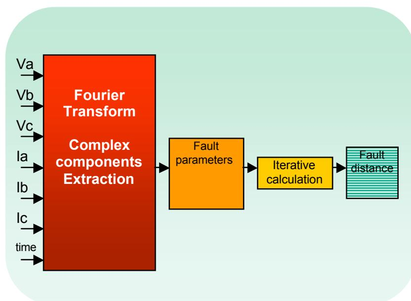
Figure 6-3 Fault distance evaluation principle
