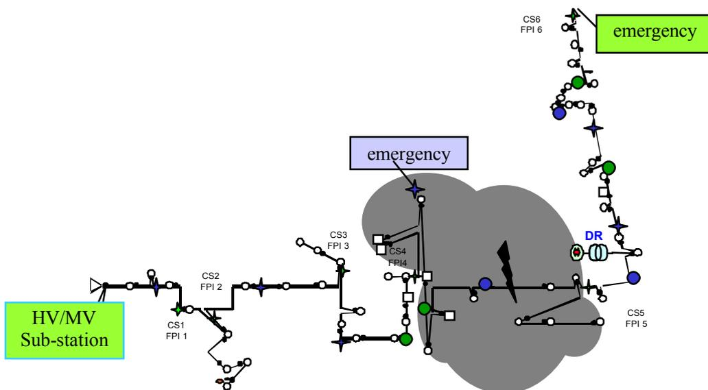
Figure 6-6 Fault localization principles step 3: faulty area reduced by remote control
