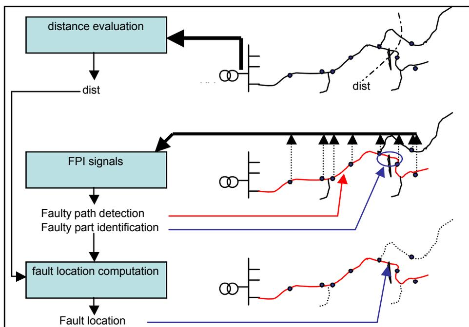
Figure 4-2 Principle for the combination of FPI and distance evaluation
