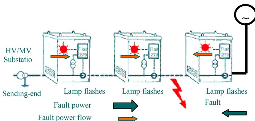
Figure 6-1 Phase directional FPI in a high DR in distribution EPS
